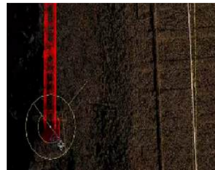
Feature extraction OHE pole
